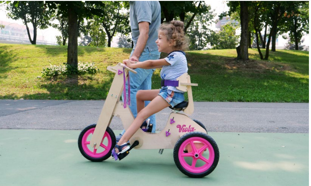
Figure 3 From the parametric file of Lorenzo's bike, OpenDot and TOG co-designed a new bike for Viola, Milan 2018
