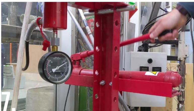
7. After 10 minutes the acrylic should be malleable and it is possible to begin to apply pressure to the mould and press the sheet.
