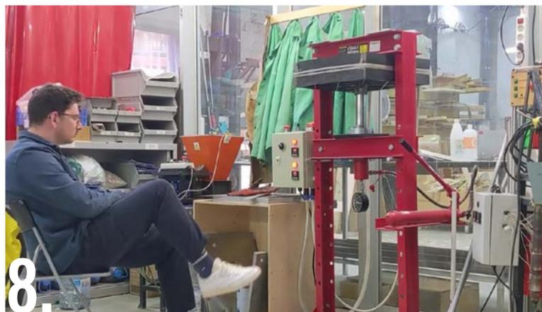
8. After the 30 minutes the pressing should be complete and it is possible to turn off the sheet press and let the machine, mould and material cool.
