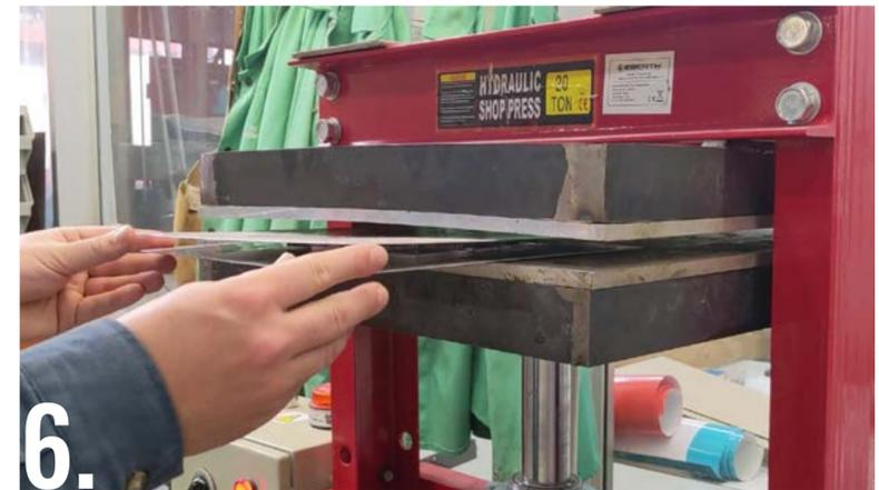
6. Place the mould into press between the heated plates and begin to bring the sheet press closed so that the plates are only just touching metal sheets and introducing heat to the acrylic to soften it.
