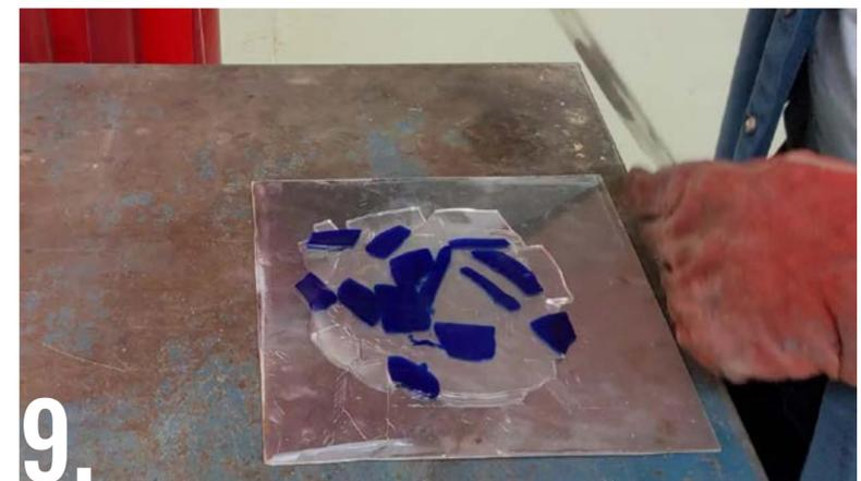
9. Once bellow 100 degrees Celsius the sheet should no longer be malleable and it is possible to remove the mould and reveal the final result.
