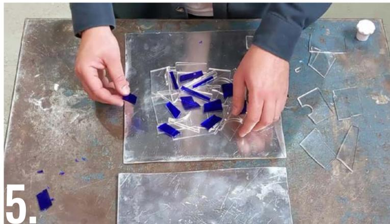
5. Prepare the mould and arrange the pieces of broken/shredded acrylic. Place the pieces with some overlap so that as they are melted and compressed together the gaps between the pieces are filled.
